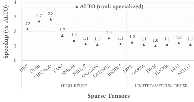
Figure 10: The speedup of ALTO using rank specialization relative to the default ALTO parallel implementation. The sparse tensors are categorized and then sorted in an increasing order of their size.
