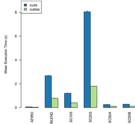
**Fig. 6.** Execution Time Comparison for Our CUDA back-end vs cuBLAS
