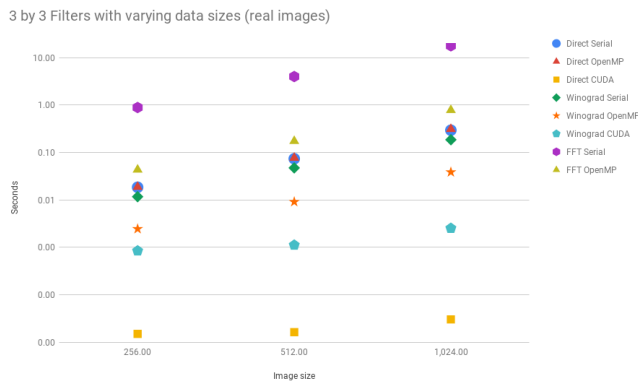
Figure 2: Runtime for real input images with size 256 × 256, 512 × 512 and 1024 × 1024 using 3 × 3 filters
